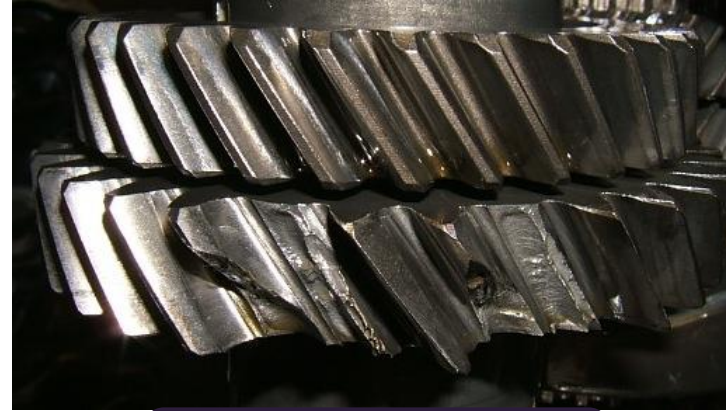
Gear Teeth Failure
